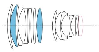
14 Elements in 12 Groups SLD (Special Low Dispersion) Glass Aspherical Lens
